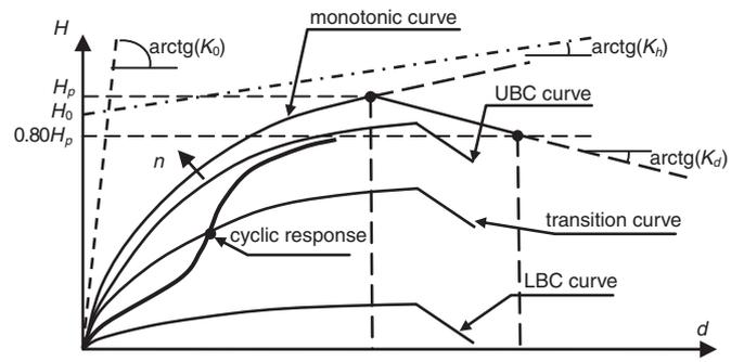
**Fig. 2.** Model of the cycle lateral response of SCFS shear walls.
