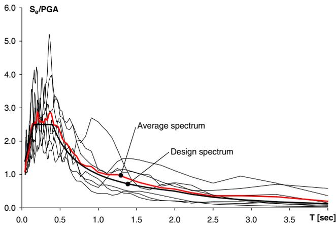
**Fig. 6a.** Eurocode 8 [4] elastic acceleration spectrum for soil type A.
