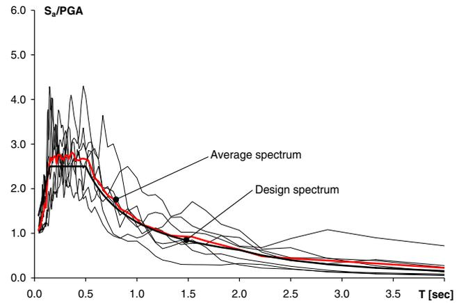
**Fig. 6b.** Eurocode 8 [4] elastic acceleration spectrum for soil type BCE.
