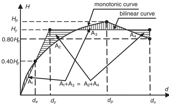
Fig. 8. Monotonic response curve of a SCFS shear wall: definition of the idealized bilinear curve.
