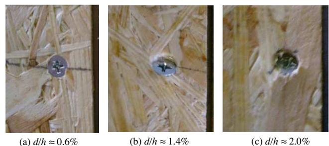
**Fig. 11.** Experimental observation of the sheathing fastener damage during a monotonic test.
