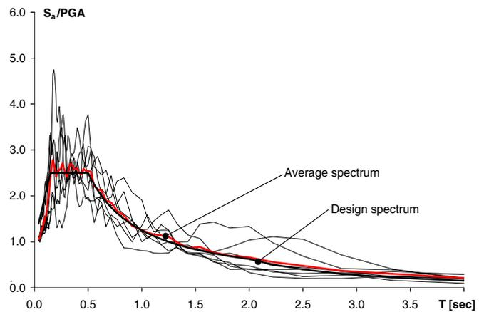
**Fig. 6c.** Eurocode 8 [4] elastic acceleration spectrum for soil type D.
