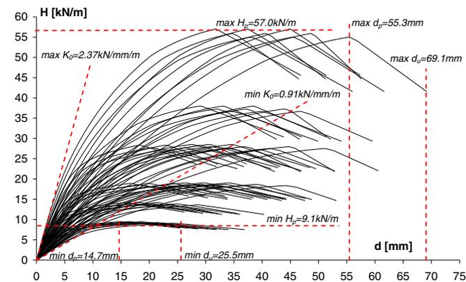
**Fig. 1.**  $H$ - $d$  response curve for all wall configurations.
