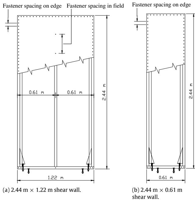
Fig. 4. Framing details for CFS shear walls for cyclic test.
