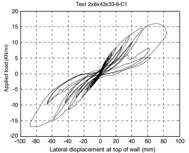
**Fig. 13.** Observed hysteresis curve for cyclic test  $2 \times 8 \times 43 \times 33-6-C1$ .
