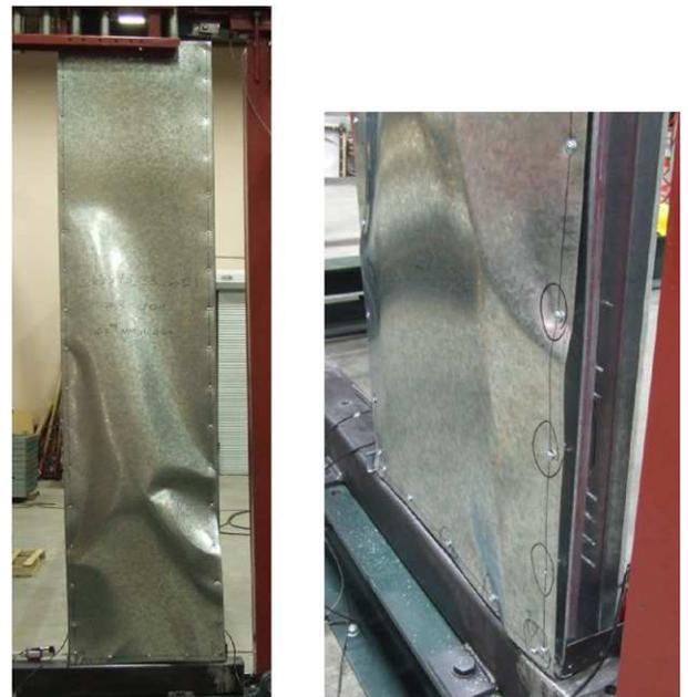
**Fig. 14.** Failure mode for test  $2 \times 8 \times 43 \times 33-6-C1$ .
