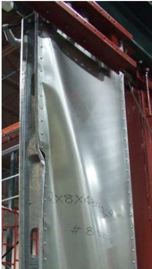
**Fig. 9.** Stud buckling on a 2.44 m × 0.61 m wall with 51 mm/305 mm screw spacing.
