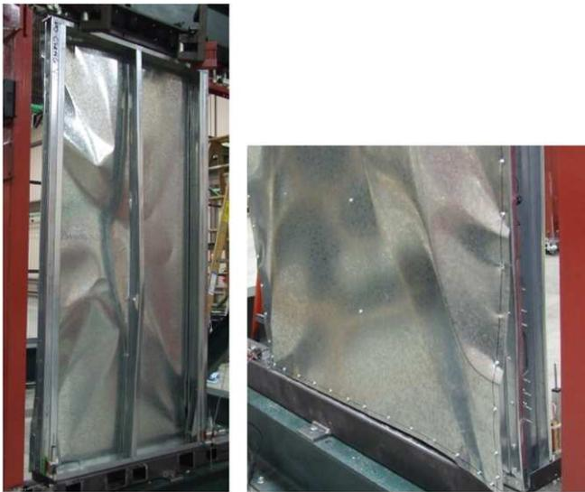
**Fig. 11.** Failure mode for test  $4 \times 8 \times 43 \times 33-4-C1$ .
