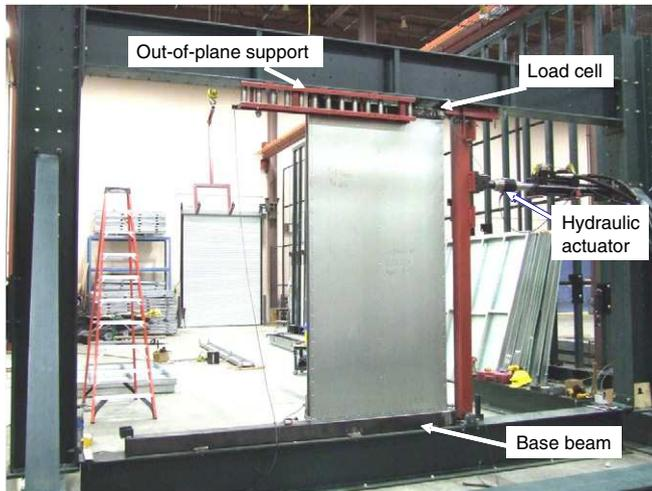
Fig. 1. Front view of the test setup.
