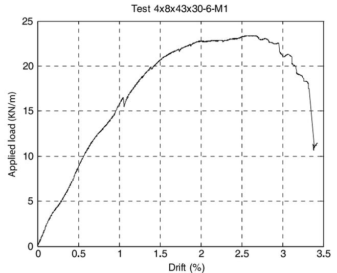
**Fig. 8.** Load vs. lateral displacement of wall top for Test 4 × 8 × 43 × 30-6-M1.
