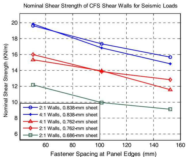
Fig. 16. Nominal strengths for seismic loads vs. fastener spacing at panel edges.
