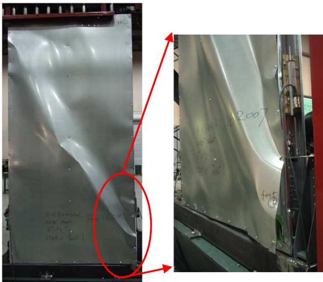
**Fig. 7.** Sheathing buckling and screw pullout on a 2.44 m × 1.22 m wall in monotonic test.
