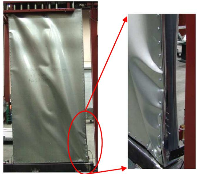
Fig. 6. Sheathing buckling and stud flange distortion on a 2.44 m x 1.22 m wall in monotonic test.
