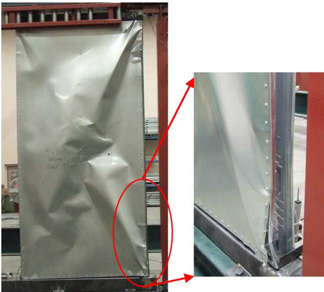
**Fig. 12.** Failure mode for test  $4 \times 8 \times 43 \times 30-2-C1$ .
