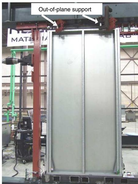
Fig. 2. Back view of the test setup.
