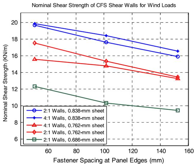
Fig. 15. Nominal strengths for wind loads vs. fastener spacing at panel edges.
