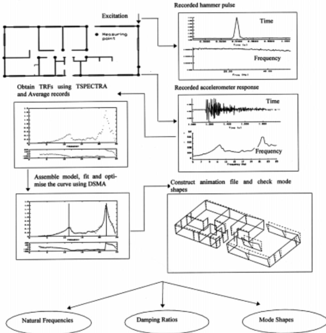
Figure 4. A summary of the modal testing and analysis procedure.
