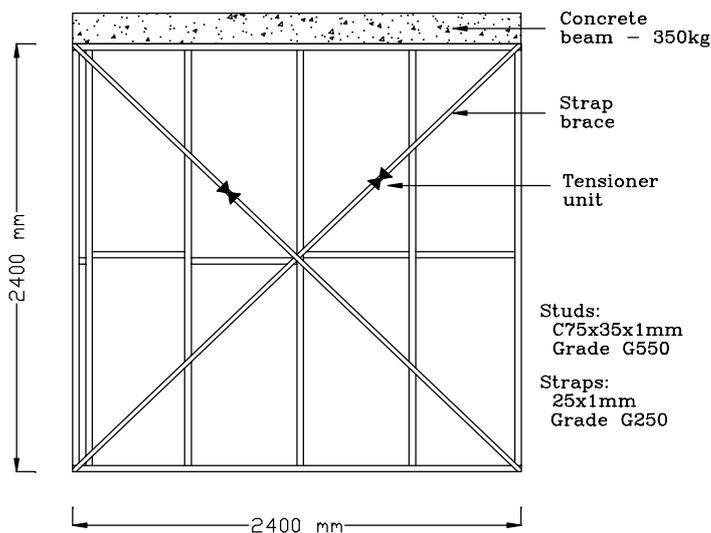
Figure 1. Typical tested isolated unlined wall frame with simulated roof mass.
