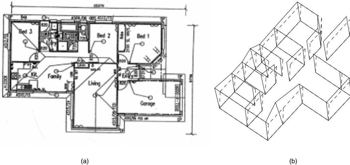
Figure 6. The Currawong floor plan and snap shot of the animated sway mode shape
