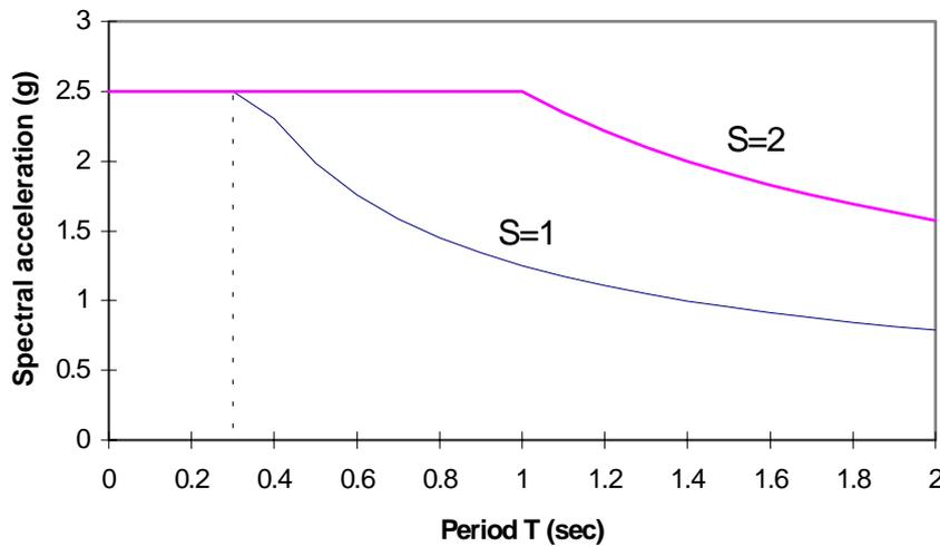
Figure 7. Normalised response spectra according to AS1170.4 showing a maximum plateau to periods up to 0.3 sec. (S=1 refers to a normal soil and S=2 refers to a soft soil).
