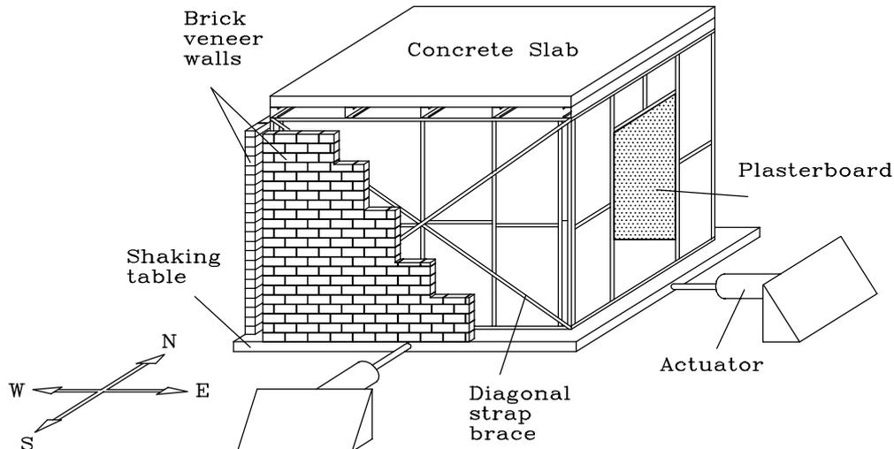
Figure 2. A schematic diagram of the test house and the shaking table.
