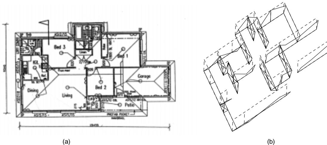
Figure 5. The Jabaru floor plan and a snap shot of the animated sway mode shape
