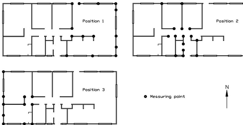
Figure 3. A typical house floor plan showing how the accelerometers are moved into three positions to cover different measuring points for excitation in the North-South direction.
