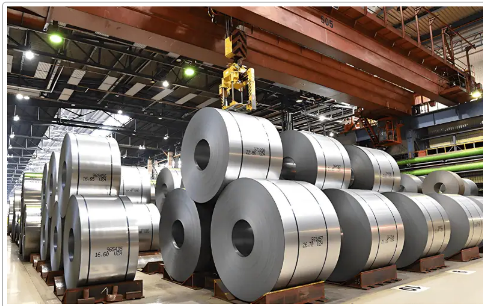
Figure: Coiled galvanized steel sheet (spangled finish) ready for roll-forming. LSF steels are specified by standardized grade and coating (e.g. AS1397/G550/AM125 or ASTM A653/G90) to ensure consistent strength and corrosion protection 2 3 .
